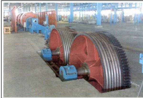
Figure (1): Photograph of Drum of Winding Machine [5].
