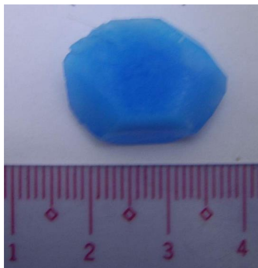
Figure 1: Photograph of the grown K_2Cu(SO_4)_2 \cdot 6H_2O single crystal.
