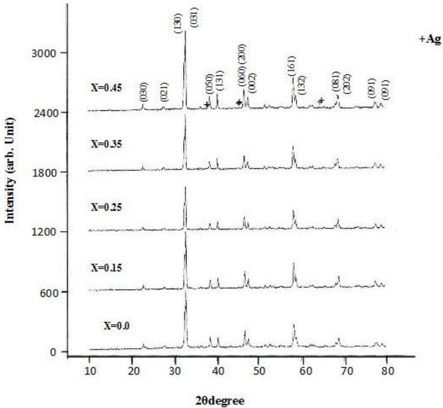
Figure (1) X-ray diffraction patterns for components  $\text{YBa}_2\text{Cu}_{3-x}\text{Ag}_x\text{O}_{6.5+\delta}$
