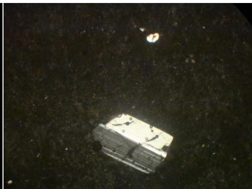
Fig. 6: Photomicrograph showing plagioclase embedded in glassy ground mass, C.N. 10X.
