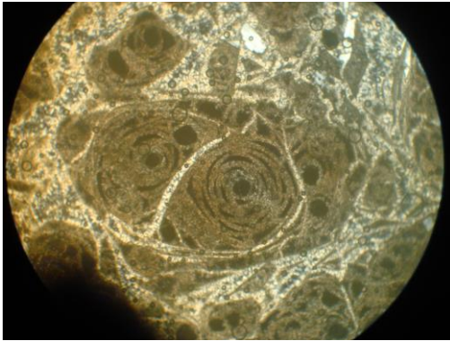
Fig. 13: Photomicrograph showing typical onion perlitic texture, C.N. 10X.
