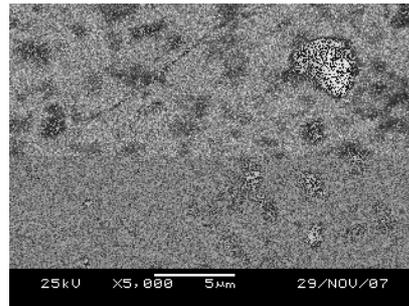
**Fig .6 (d). Irradiated HDPE/Mg(OH)<sub>2</sub>/TCA-27**
