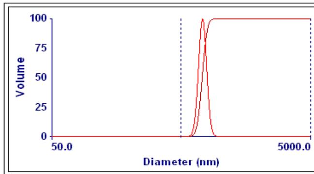
Fig.1. Particle Size Distribution of  $\text{Mg}(\text{OH})_2$
