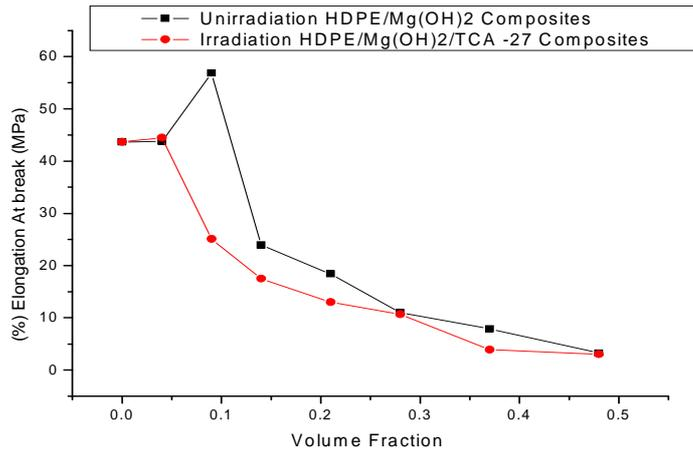
**Figure 3 : ( % ) Elongation at Break as a Function Volume Fraction of HDPE/Mg(OH)<sub>2</sub>/TCA-27 Composites .**
