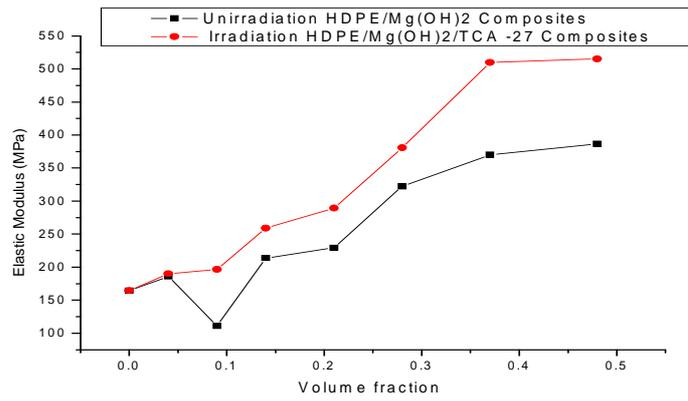
**Figure 5 : Elastic Modulus as a Function Volume Fraction of HDPE/Mg(OH)<sub>2</sub>/TCA-27 Composites.**
