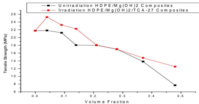
**Figure 2: Tensile Strength as a Function Volume Fraction of HDPE/Mg(OH)2/TCA-27 Composites.**
