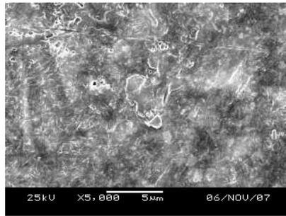
**Fig .6 (c). Unirradiated HDPE/Mg(OH)<sub>2</sub>**
