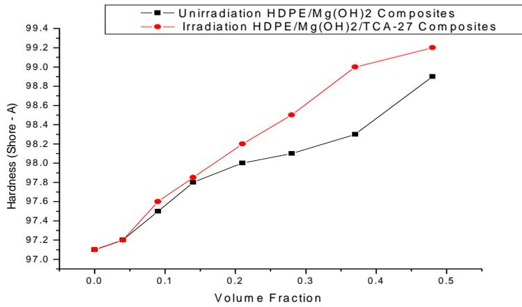
**Figure 4 : Hardness as a Function Volume Fraction of HDPE/Mg(OH)<sub>2</sub>/TCA-27 Composites.**
