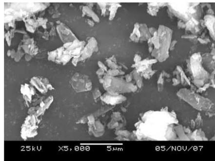
**Fig .6 (a) : SEM of Mg(OH)<sub>2</sub> Powder (200nm) .**
